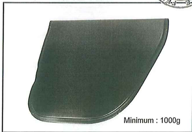
Rear side protection panel, dismantled
