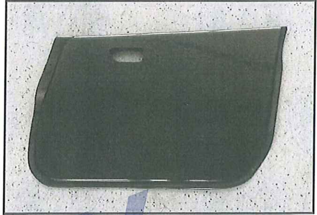
Front side protection panel – cut out option 2, dismantled
