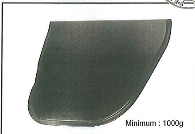
Rear side protection panel, dismantled
