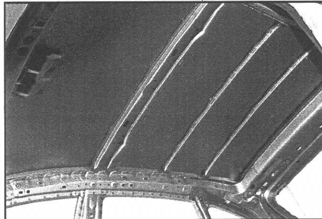
N1-6) Châssis nu – Toit vu de l'habitacle Bare chassis – Roof seen from cockpit
